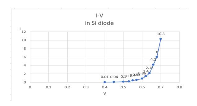
This is a graph for Si diode. And we conclude from the figure that the relationship is non-linear.
