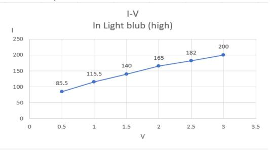
This is a graph for Light bulb (high). And we conclude from the figure that the relationship is non-linear.
