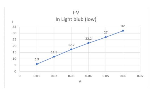
This is a graph for Light bulb (low). And we conclude from the figure that the relationship is linear.
